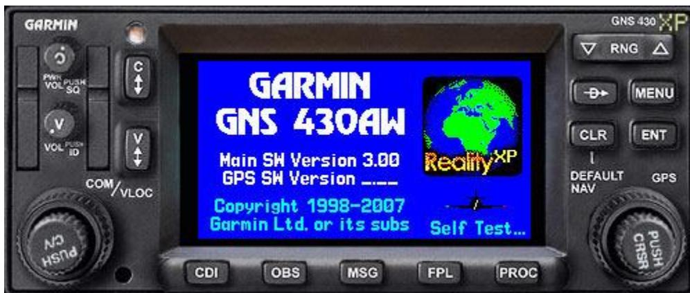
ILS approaches are not labeled ILS or GPS (RNAV). An ILS approach must use the ILS signal. The GPS does a great job on the map with the localizer line and the various fixes for orientation and situational awareness. Therefore, during an ILS approach, the CDI Mode must be switched to "VLOC" instead of "GPS".
