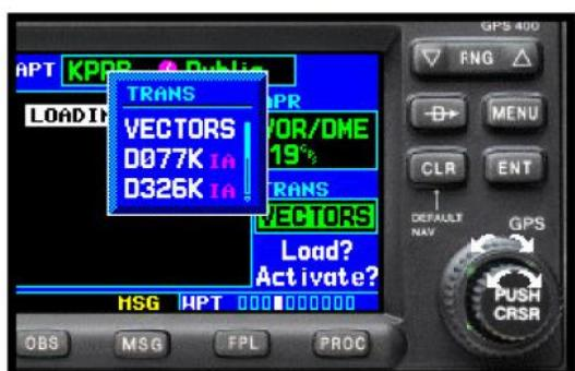
Selecting an IAF can be a bit confusing. Instead of spelling out JEBNO and YERGU, the GNS uses the radial and D (DME). JEBNO is on the 077° Radial and YERGU is on the 326°R. "K" indicates the 11 DME arc. See next paragraph for explanation.
