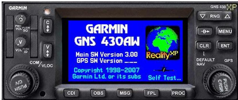
Press the **PROC** button, and using the LARGE and small knobs, choose the desired approach.
