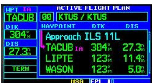
If you have loaded the ILS with "Vectors to Final", and subsequently, ATC clears you direct to TACUB and the ILS approach . . .
